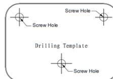
3. Use 3 screws to fix the bracket to the ceiling and the screw hole on the bracket should align with the mounting hole on the drill template.
